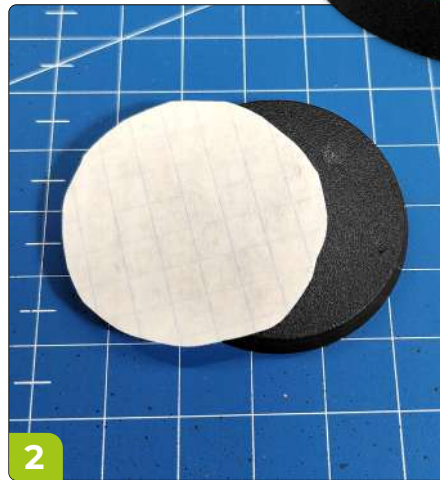
2. Using a 40 mm paper template I cut the photo-etched plate to the correct shape.
